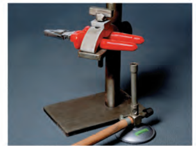
Testing of flame resistance
