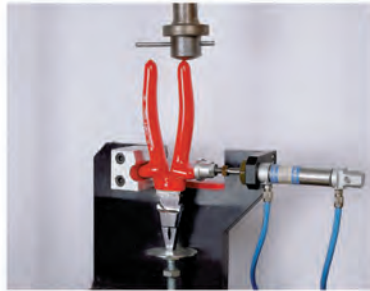
Cold impact test
